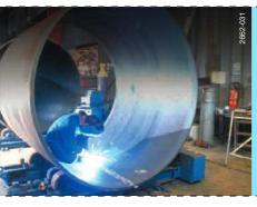
Easy-to use line of rotators covering a load carrying range from 2 tons up to 600 tons (Drive unit + Idler unit).
